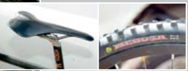
SID'S XC RACER - Sid Taberlay's carbon fibre Avanti hardtail. Note the Selle Italia SLR saddle with the leather and padding removed. The ultra-skinny 1.55 tyres were a typical wet weather choice, just in case the sky's opened up.
