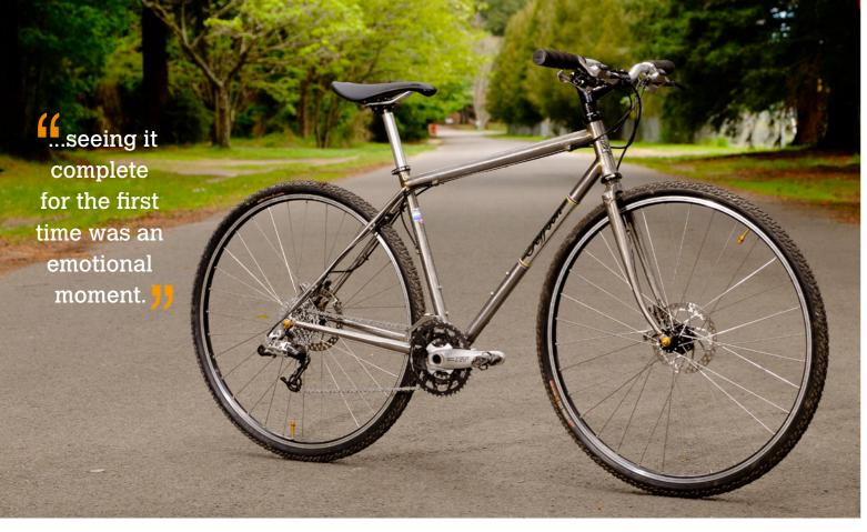
also used rods of 24% silver to braze on the cable runners. Silver has a significantly lower melting point than bronze and the torch was set no higher than the flame on a kitchen gas hob.
